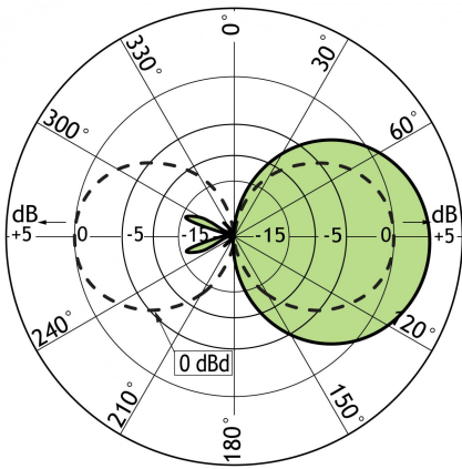
This curve shows the radiation patterns in the vertical plane.
