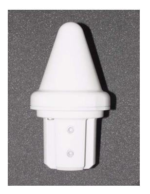
The L1GPSA-N GPS antenna is a 38db Gain Antenna designed specifically for the GPS L1 carrier frequency. The L1GPSA-N is powered by 5VDC it receives on the center conductor.
